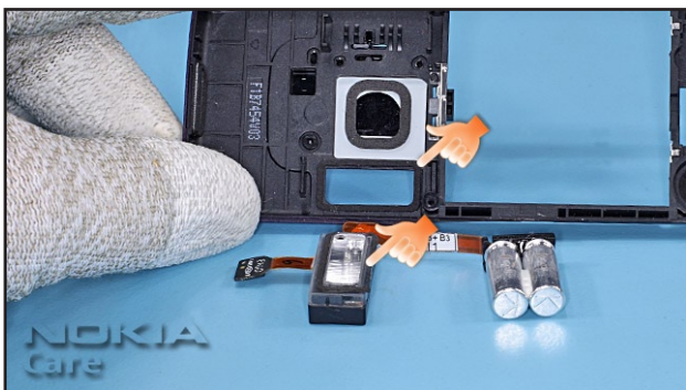
3. Attention - Please read the Handling instruction in the chapter 3. Warnings & Cautions. Take special care to the flex when Remove the adhesive residues. Use always a new FLASH LIGHT GASKET when re-fitting the FLASH.
