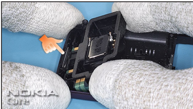
5. Fit the ANTENNA BOX paying attention to the IHF gasket.
