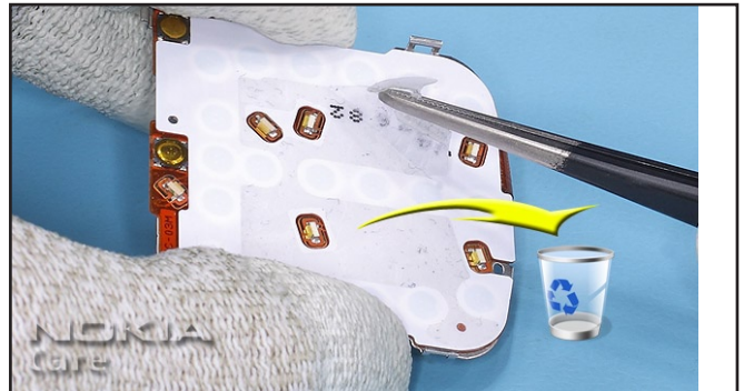
26. In case the KEYMAT has been removed more than two times or the keymat adhesive is even slightly dirty or dusty, remove the KEYMAT ADHESIVE paying attention to the LEDs and discard it.
