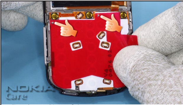
9. Align the markings of the new KEYMAT ADHESIVE with the UI ASSY. Ensure that the ADHESIVE is glued well and carefully remove the carrier foil.
