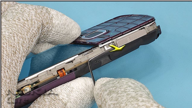
9. Unlock all snaps of the UI SHEET ASSY with the dental pick.
